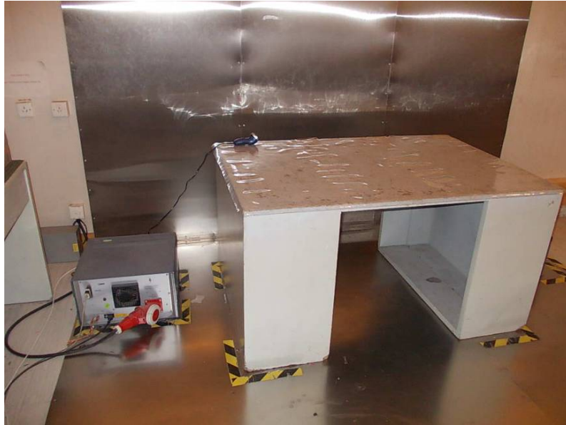
Figure 2 Conducted Emission test setup
