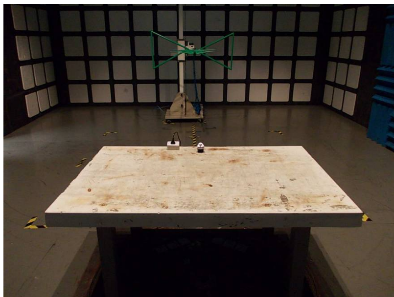
Figure 3 Radiated emission test setup
